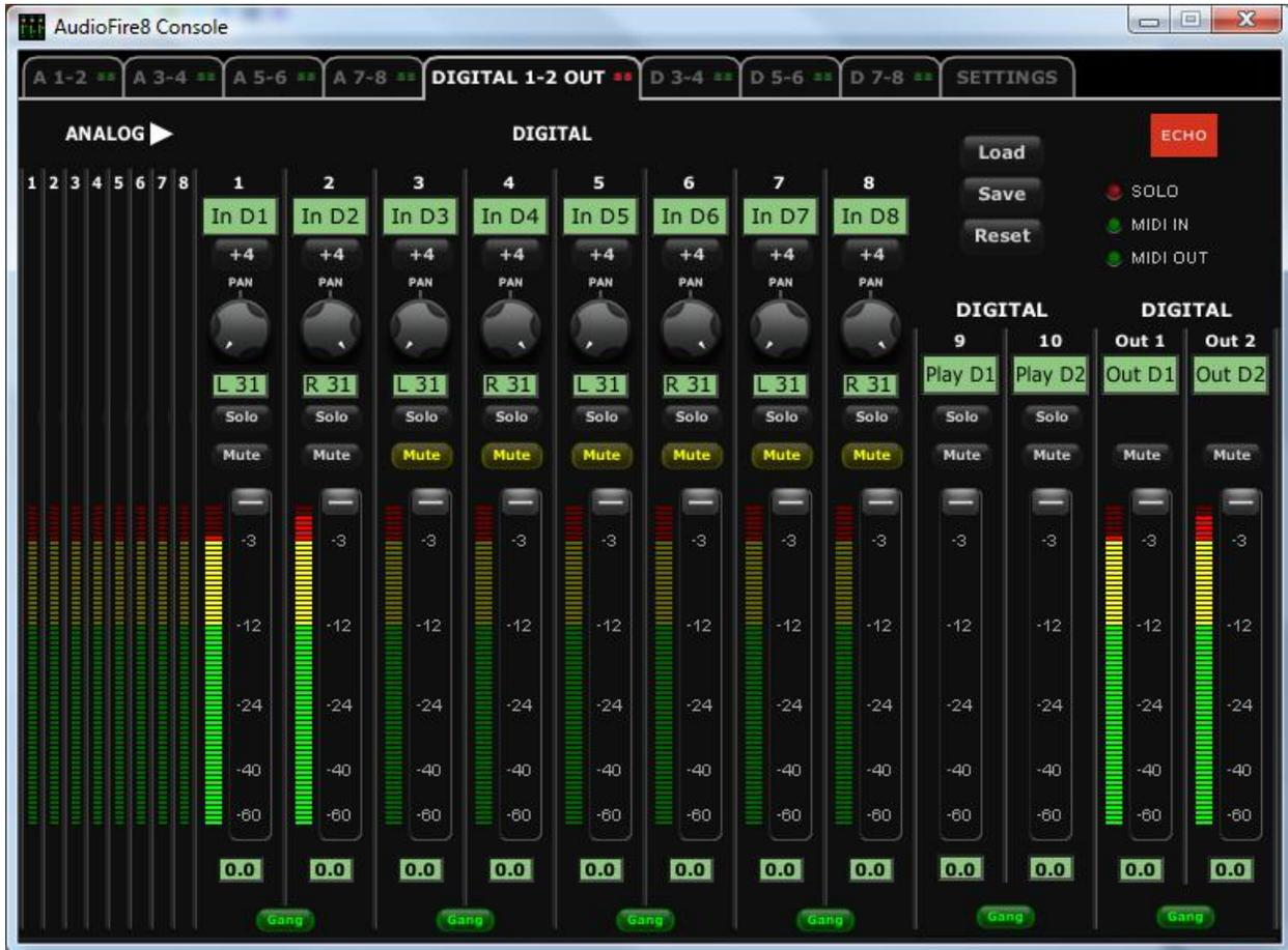
*AF 8 Console Window on Vista: Digital Out 1-2 Tab selected (expanded view).*
