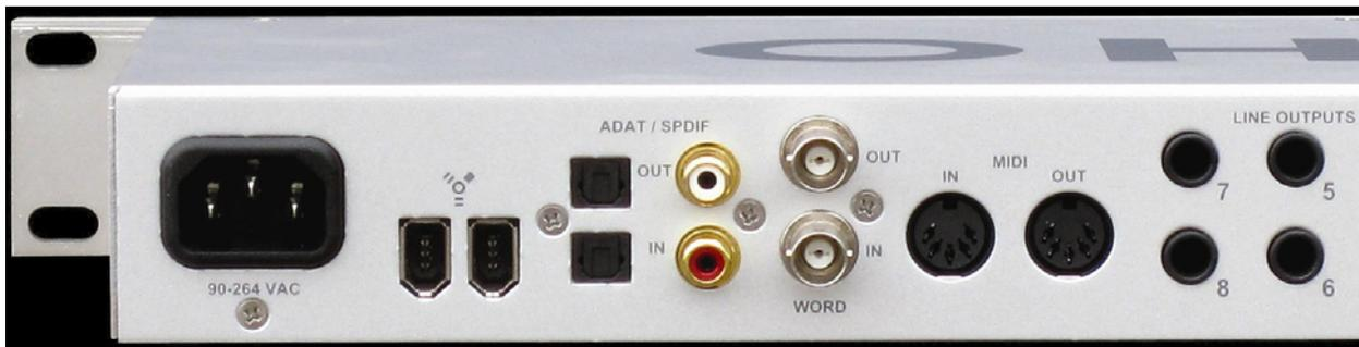
The rear panel has universal inputs 3 – 8, line outputs 1 – 8, 2 channel inserts, MIDI i/o, S/PDIF i/o, ADAT i/o, BNC WordClock connectors, and two FireWire connectors.
