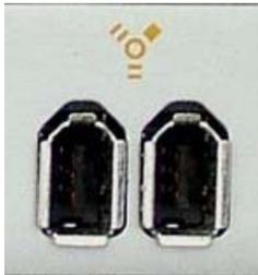
**Caution:** Plugging the FireWire cable in rotated 180 degrees can cause permanent damage to your AudioFire, FireWire adapter, or both. Make sure the cable is oriented correctly with the angled edges of the plug matching the angled edges of the socket. Plug the cable straight in. Do not force. It is recommended that FireWire connections be made when the computer is turned off.
