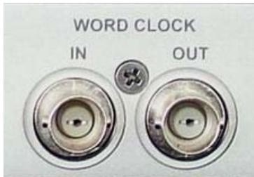
The Word Clock I/O uses a BNC connector. As with the S/PDIF I/O, a shielded 75-ohm (RG-59) coaxial video cable should be used. BNC connectors have been widely used in the electronics industry for both video and computer networking. However, computer networks use 50-ohm (RG-58) coaxial cables and not the 75-ohm (RG-59) cable used by video. For reliable word clock operation, use only video grade cables with your Echo product.
